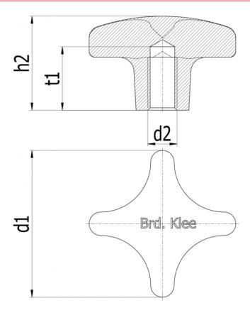
$\begin{array}{lll} d1 & = 32 \\ d2 & = M6 \\ h2 & = 20 \\ h4 & = 9 \\ t1 & = 12 \\ Weight in (g) = 38 \end{array}$
